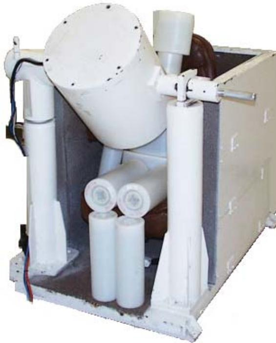
**Whole body counting chair and detector system used to test for presence of cesium-137 (radiocesium) inside peoples' bodies.**
