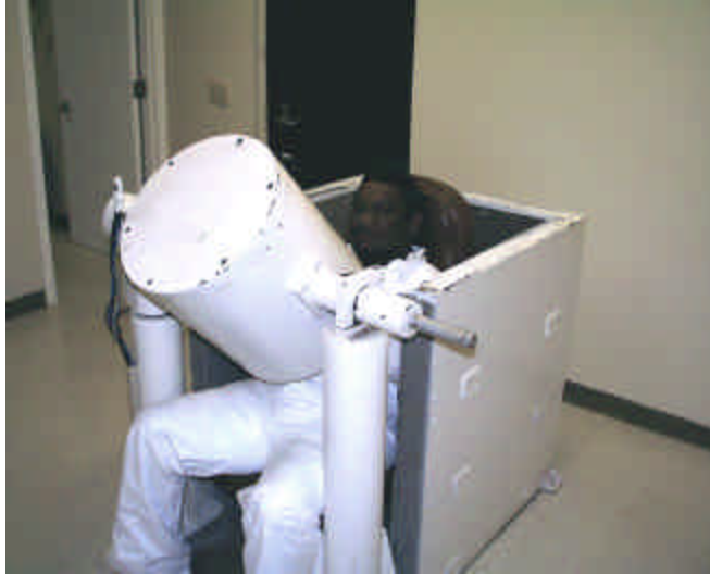
Figure 4. The Rongelap whole-body counter with a volunteer seated in the chair.
