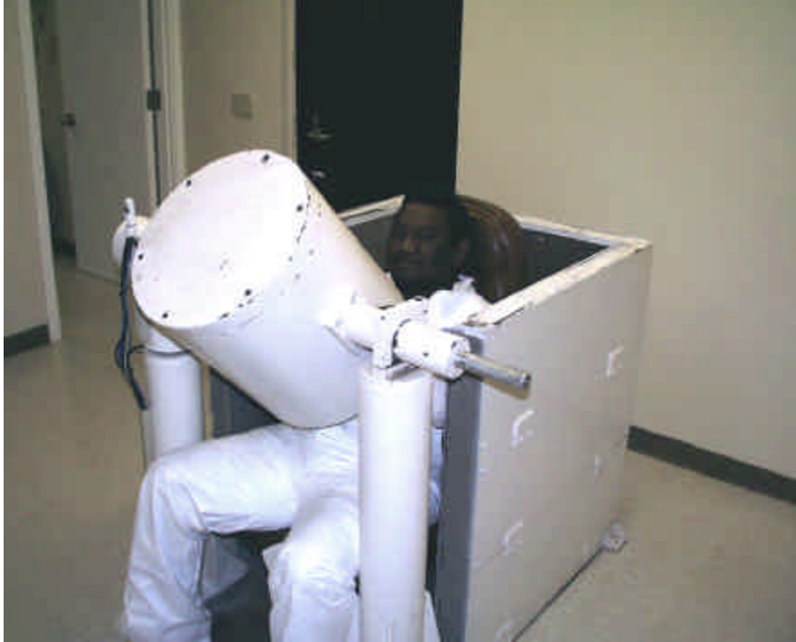
Figure 3. The whole-body counter with a volunteer seated in the chair.
