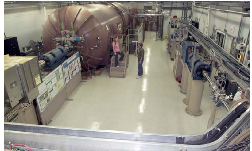
HVEC Model FN Tandem Van de Graaff accelerator operated at voltages up to 9 MV: gas or foil stripping
