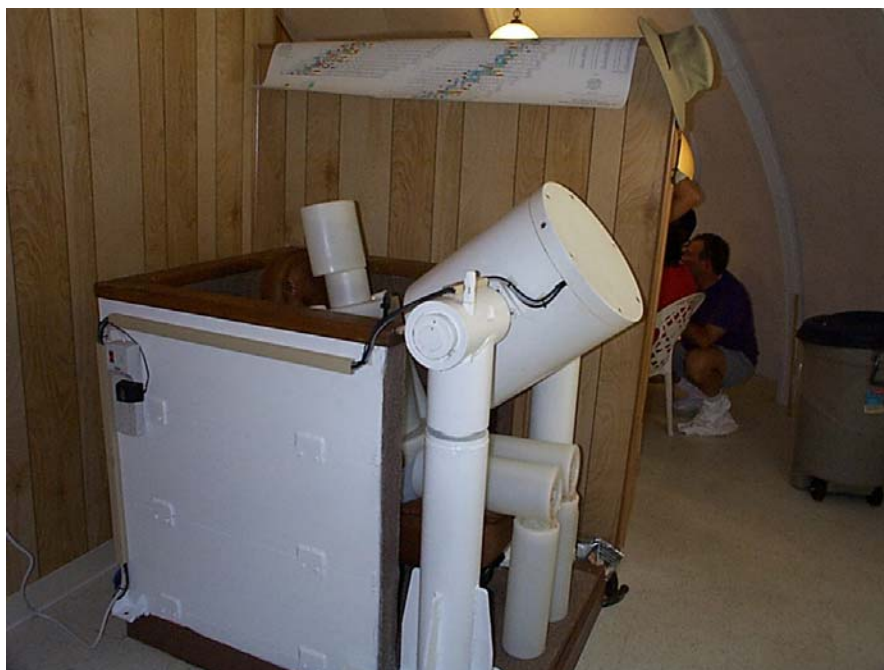
Figure 3. The Enewetak Radiological Laboratory whole body counter with a plastic calibration phantom seated in the chair.
