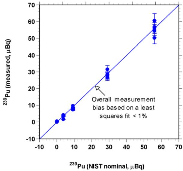
**Figure 2.** Results of the NIST intercomparison exercise on low-level plutonium isotope measurements in a synthetic urine matrix.
