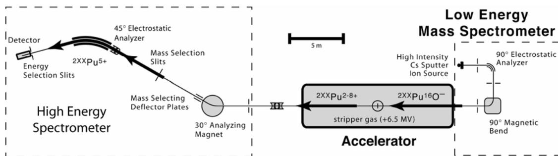
**Figure 1.** Outline of the heavy isotope accelerator mass spectrometry system at CAMS.
