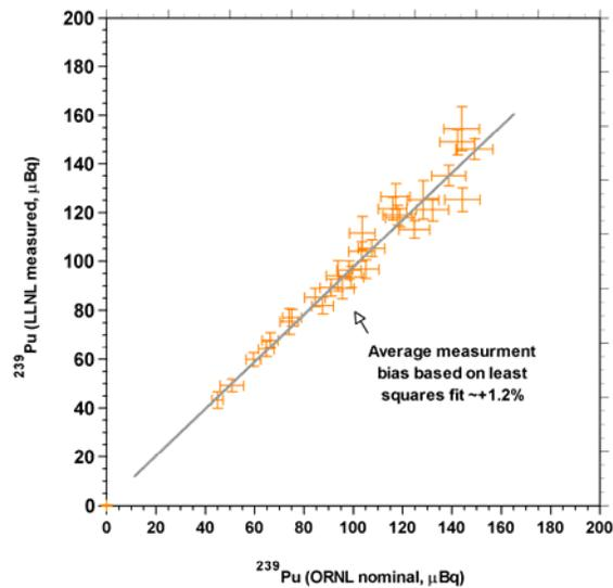
**Figure 3.** Results of  $^{239}\text{Pu}$  measurements in externally-prepared natural matrix spiked bioassay (urine) Quality Control samples.
